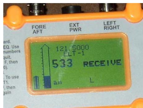
Figure 5. L-Per<sup>®</sup> Operating Screen in the Receive Mode.
