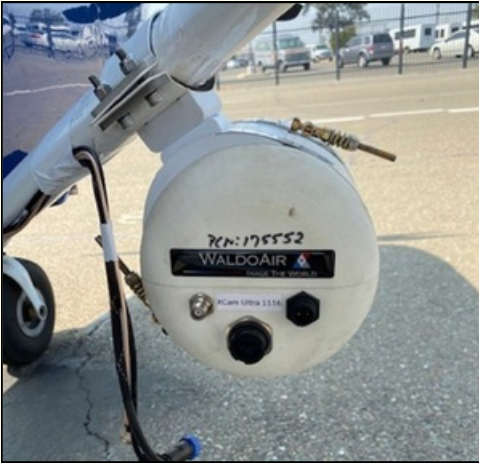
Figure 1 - WALDO camera system installed on a C182. Photo Credit: Lt Col David Rudawitz
